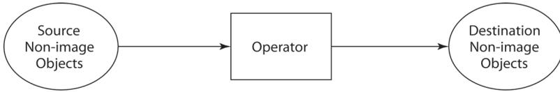
**FIGURE 1.1-3.** PIKS operator model: non-image to non-image operators.
